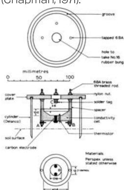
Fig. 1. Constructional details of respirometer
