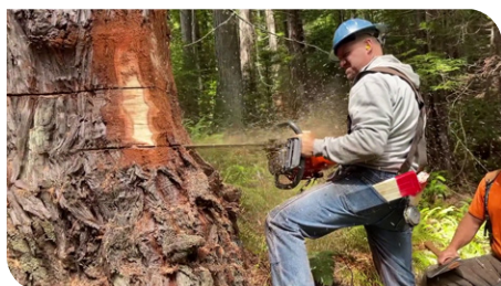
Figure 24: Video 2, 12:38. Horizontal use projecting debris toward the user.
