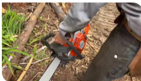
Figure 25: Video 2, 02:58. Dangerous drop starting technique is used.
