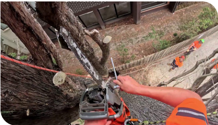
Figure 20: Video 1, 6:55. Correcting chain tension while in the crown.
