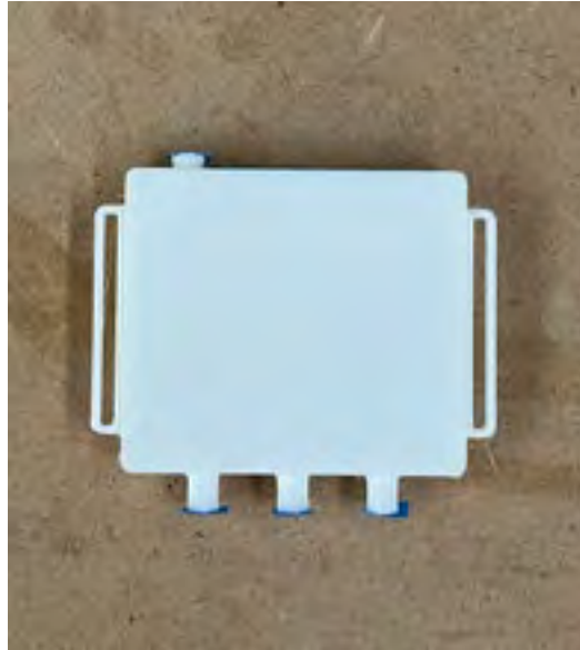
Components prepared by taping holes and areas not wanting to be painted
