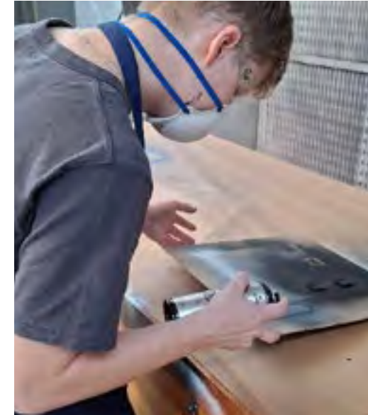
Spray painting parts in context using water based spray paint and cardboard plates
