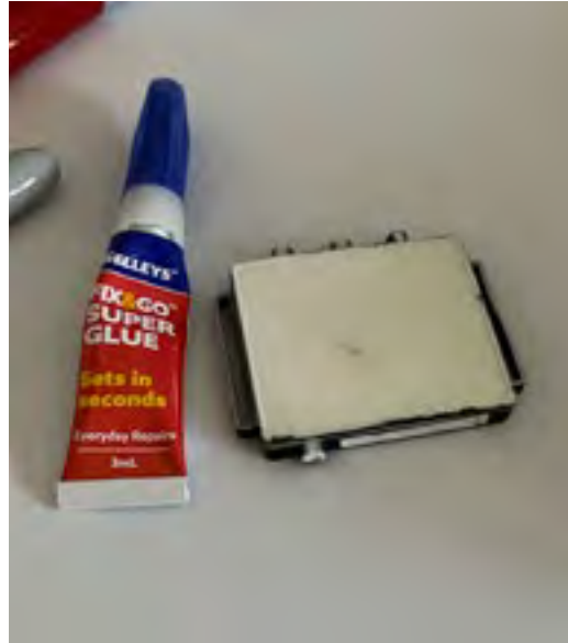
Interface screen and interface compartment joined together
