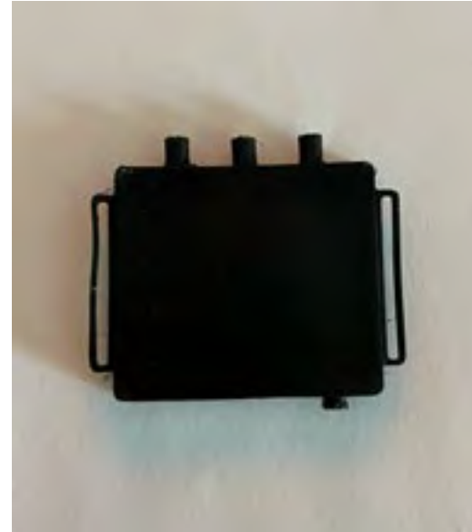
Full coated and glued interface compartment and screen ready for assembly
