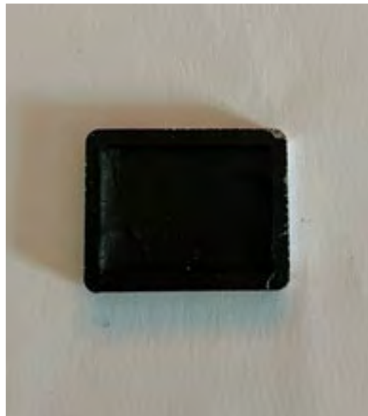
LED panel screen prepared by covering areas with tape and spray painting edges
