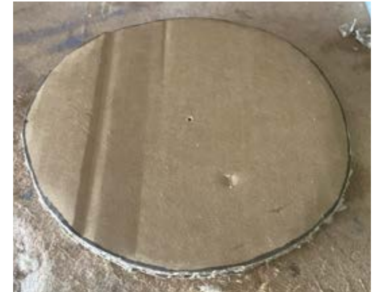
Main body was traced and cut in a circle
