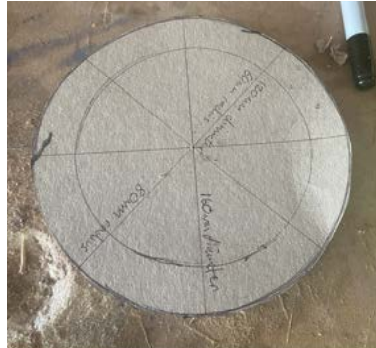
A circle containing measurements of the main body and rotating sectors was drawn up.
