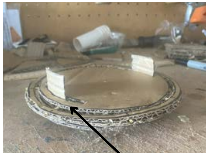
Two small corrugated cardboard strips were cut and attached to the base of the "light" part as attachment pieces.
