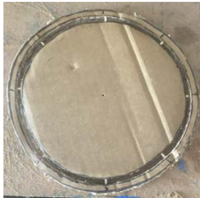
Eight toothpicks were inserted into the ring and main body to connect the two together safely and securely.
