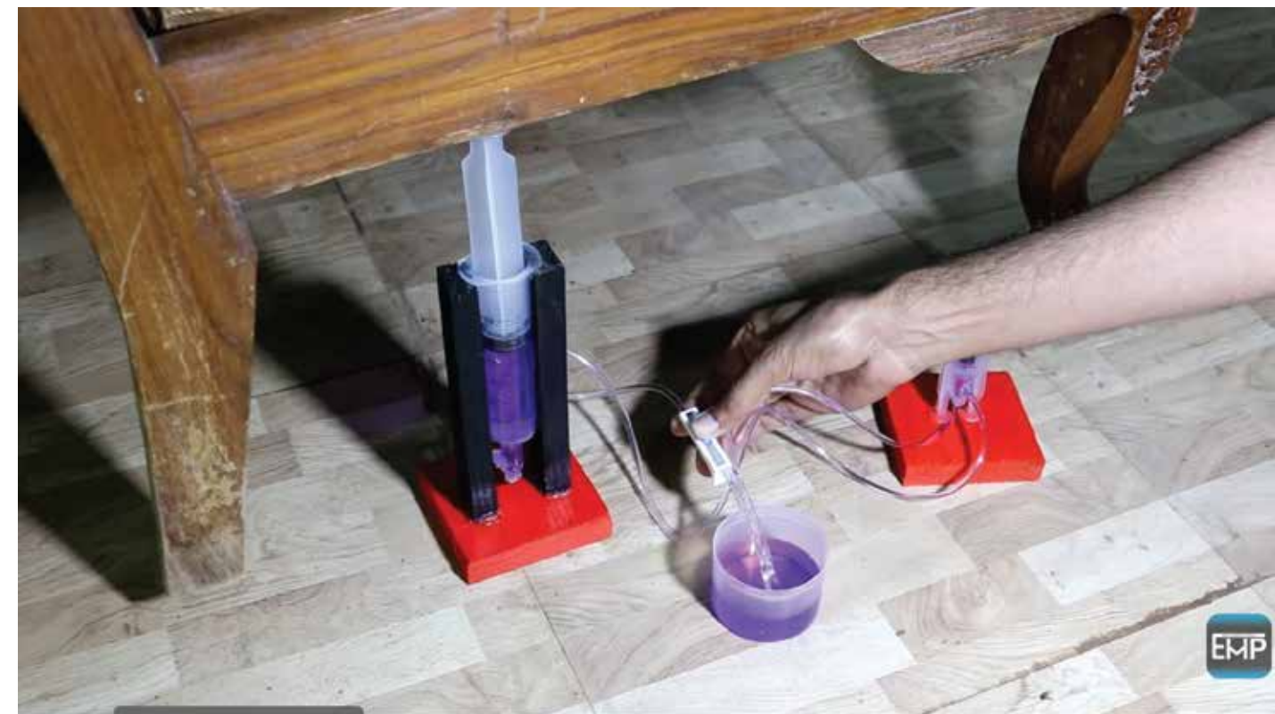
How to Make a Powerful Hydraulic Jack using Syringe
