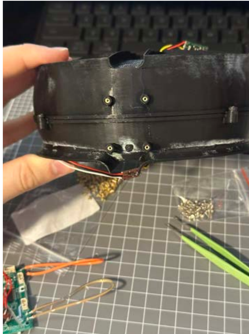
PCB is attached via heat threaded inserts, which are set in the 3d print plastic via a soldering iron
