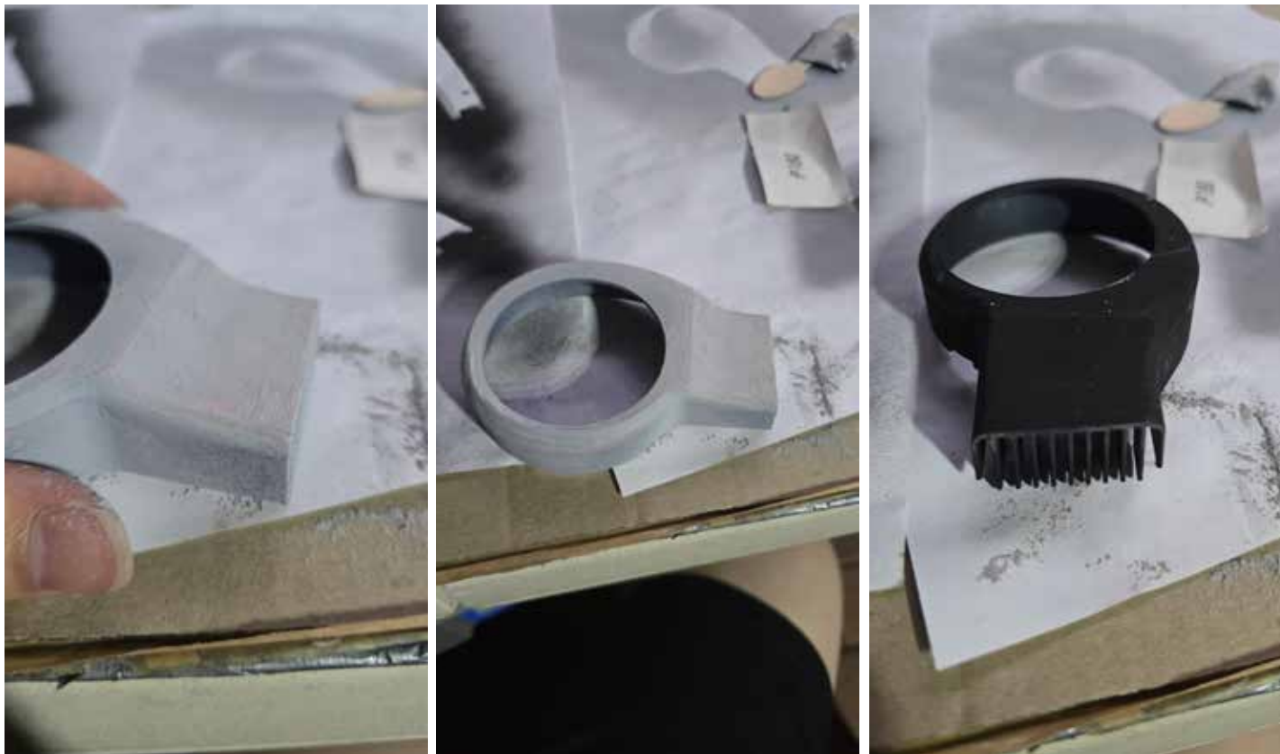
Filled large gaps with blade putty, primed then sanded down
