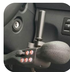
Figure J: Adjustable lever for acceleration and button controls ( Trigger Accelerator and Brake Lever | Total Ability Australia )
