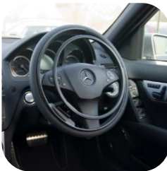
Figure F: Steering wheel additive that moves acceleration/deceleration to hand controls ( Hand and Driving Controls for Vehicles - Mobility Engineering, 2024 )
