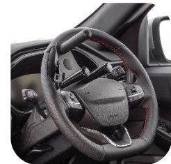
Figure H: Steering wheel adapter for reduced grip users ( Steering Aids for Assisting with Driving | Jeff Gosling, 2025 )
