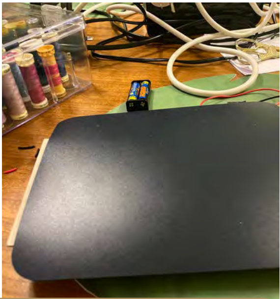
Testing with a vinyl covering. It was found that the vinyl covers which had a bit of texture on them were the most effective for transmitting the vibrations to the user. The vibration could be felt on the lower arm and the hands/ wrists.,
