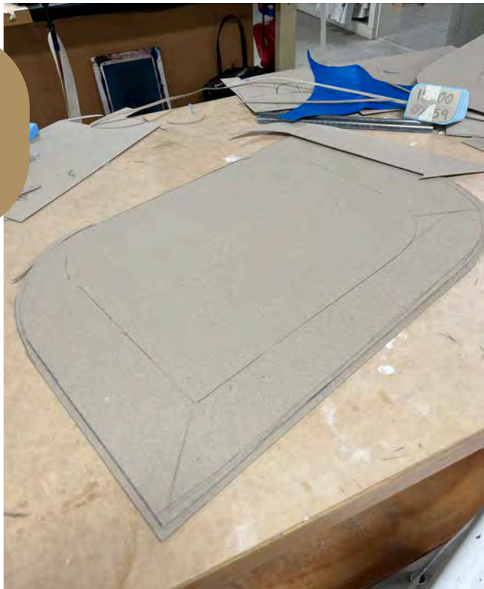
In the final design, there should be a separate centre piece which follows the same line but offset. This is so that there is an internal piece that is less affected by the vibrations for the laptop to sit on. It also means that there will be channels created for the electrical wiring of the piezos in the model.
