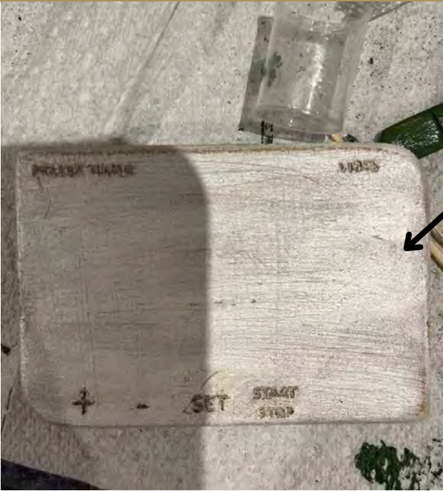
The button control panel was laser cut then sanded down to round the edges. The labels 'preset timer,' 'vibes,' and custom setting symbols were engraved. These would be embossed if mass manufactured.
