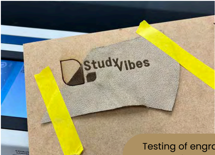
Testing of hand-colouring the faux suede. This did not look clean, therefore the taupe colour will be used, with an engraved logo.
