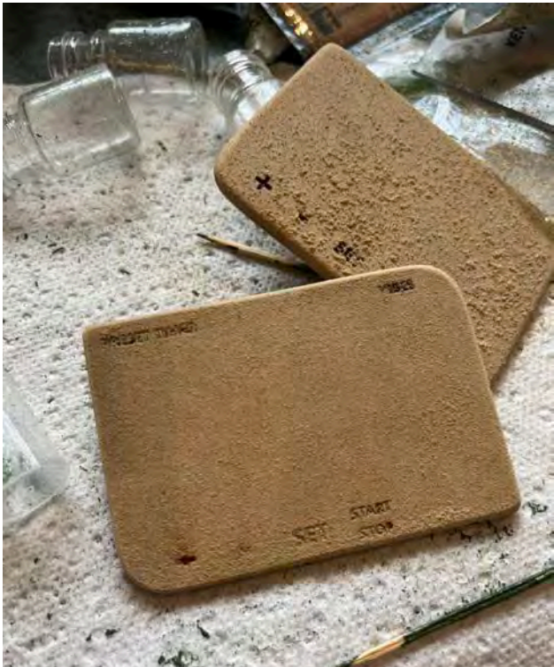
The button control panel was laser cut then sanded down to round the edges. The labels 'preset timer,' 'vibes,' and custom setting symbols were engraved. These would be embossed if mass manufactured.
